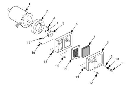
Figure 21 - Motor and Pump Assembly
